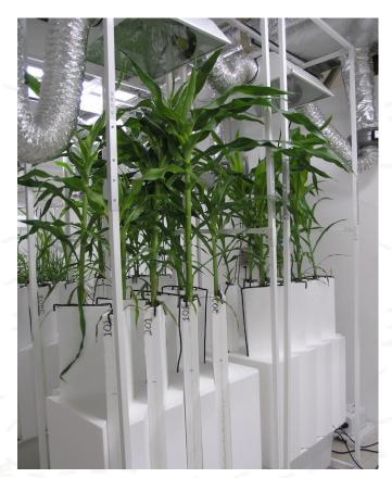
Plant containers are available in a range of sizes and may be custom manufactured in a size to suit the experimenter's needs. We presently provide sizes from our smallest container of 30x50x200 mm (used primarily for early root emergence and seed treatment evaluation studies) up to the largest container of 45x200x1000 mm (used for larger plant species and longer duration experiments.)
