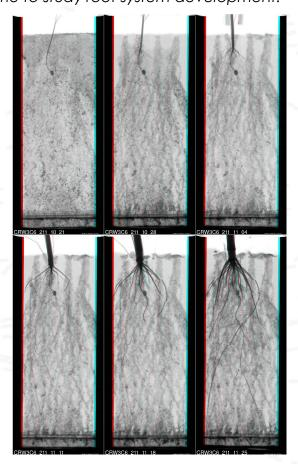
For non-destructive imaging the plant is grown in our Root Lab in a plant container and a growth substrate selected for supporting healthy plant growth and for very low X-ray attenuation properties. This combination allows imaging and analysis of the entire root system and opens new possibilities for phenology studies.
