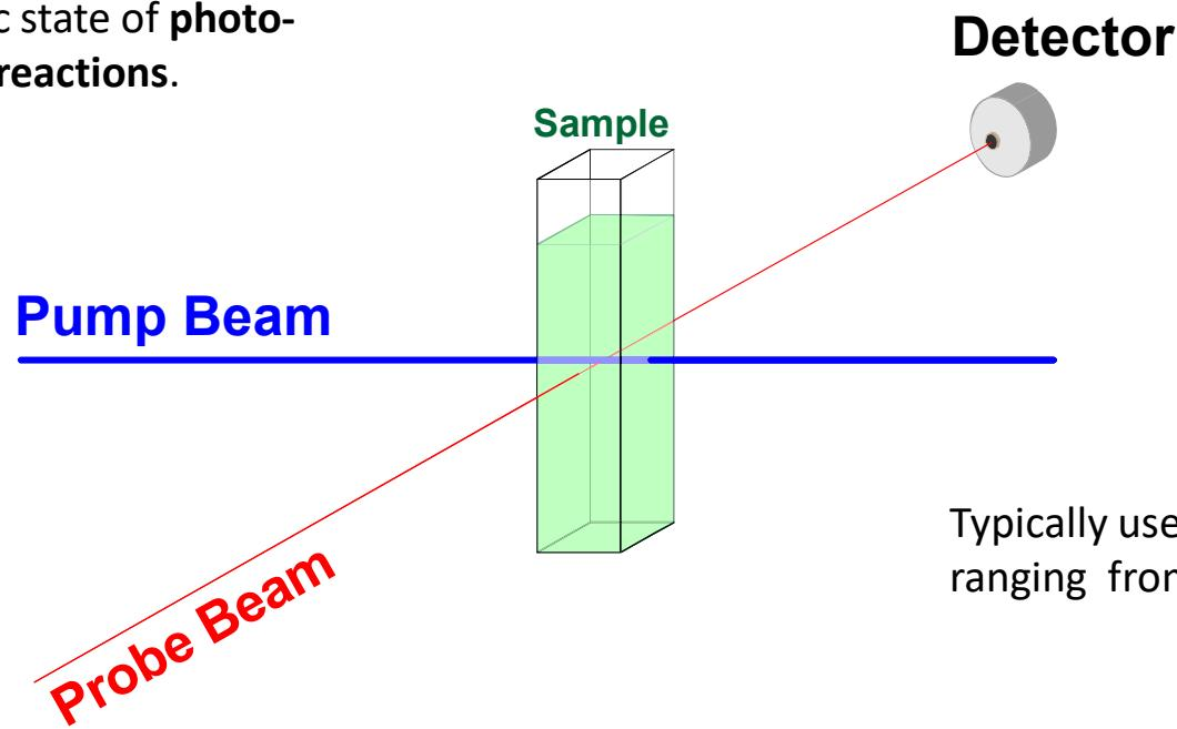
Typically used to measure rates ranging from  $10^{12} - 10^6 \text{ s}^{-1}$ .
