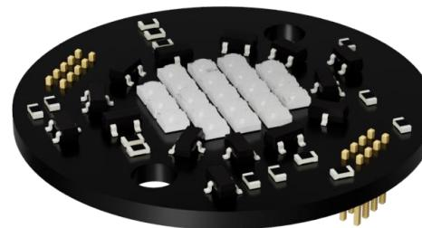
LED board with FETs for fast switching
