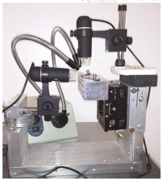
Figure 2. Droplet Characterization systems consists of two perpendicular video cameras which capture droplet spread over leaf surface.
