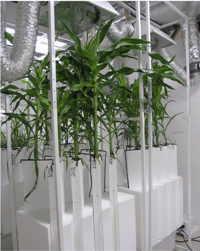
Plant containers are available in a range of sizes and may be custom manufactured in a size to suit the experimenter's needs. We presently provide sizes from our smallest container of 30x50x200 mm (used primarily for early root emergence and seed treatment evaluation studies) up to the largest container of 45x200x1000 mm (used for larger plant species and longer duration experiments.)
